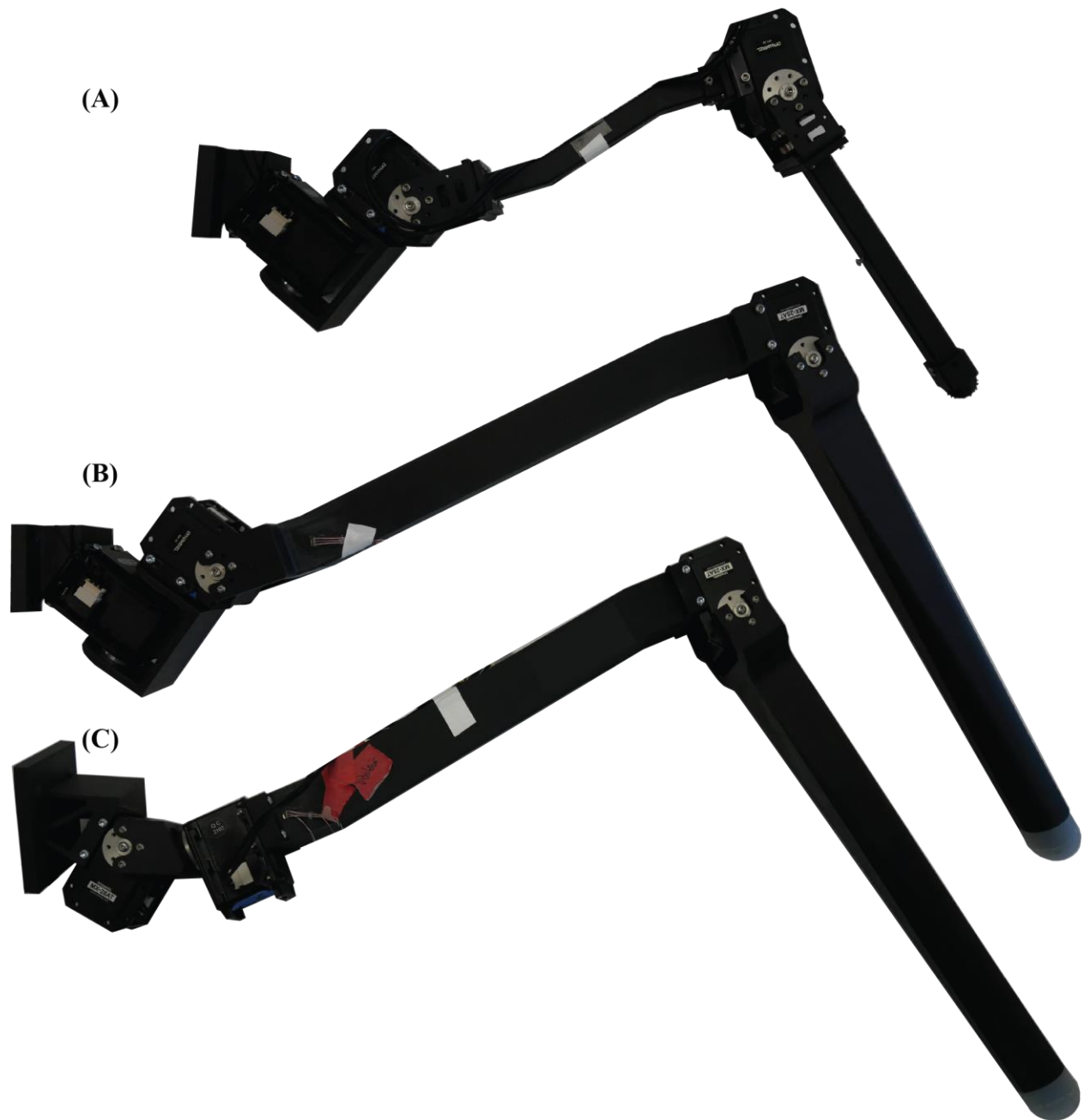
Figure 4: Robotic Leg Pictures. (A) C. morosus 15:1 scaled leg, (B) C. morosus 25:1 scaled leg, (C) D. melanogaster 400:1 scaled leg
