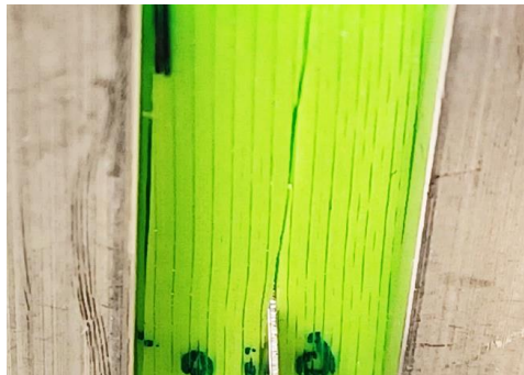
Figure 34. Scalpel cross cutting parallel print layers of the specimen.
