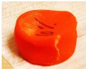
Figure 22. Buckled specimen after confined compression testing.
