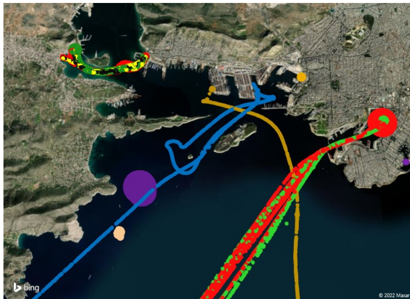
Figure 1.3: Visualization of vessels and associated tracks in the AIS dataset. Each color corresponds to a track from a different vessel. The map demonstrates the overlapping of the tracks of vessels which makes the track association problem challenging
