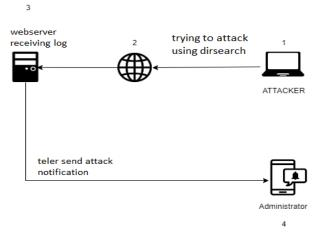
Figure 1. System Architecture
