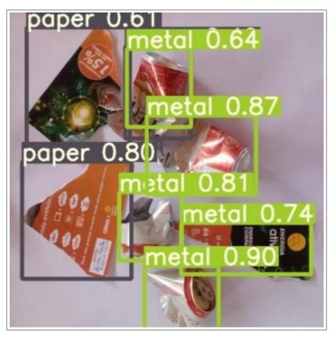
Figura 1. Example of the process of detecting and classifying discarded waste
