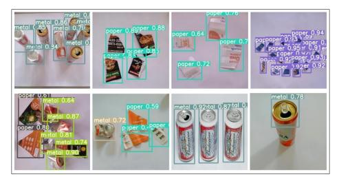
Figura 5. Objects classified in the paper and metal categories, and the level of accuracy resulting from running YOLOv5
