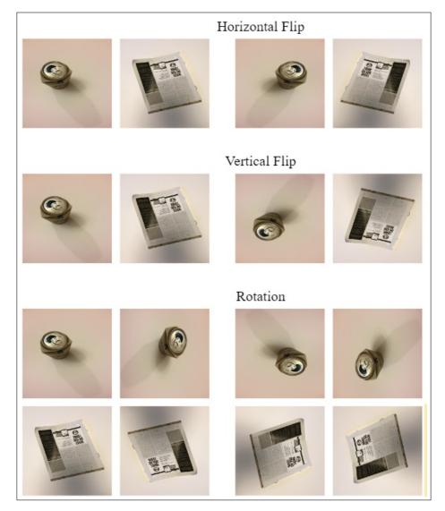
Figura 2. Modifications applied to the original images: horizontal flip, vertical flip, and rotation
