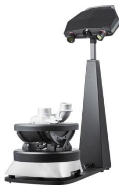
Figure 4. The used 3D scanner (Solutionix C500)
