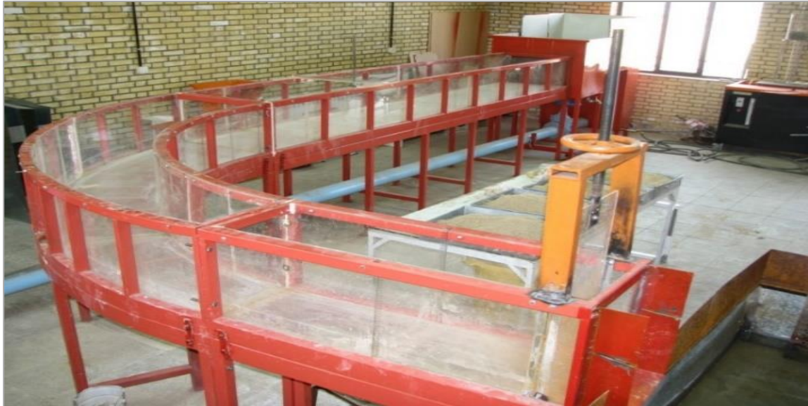
Figure 3. Laboratory physical model with a 90° convergent bend
