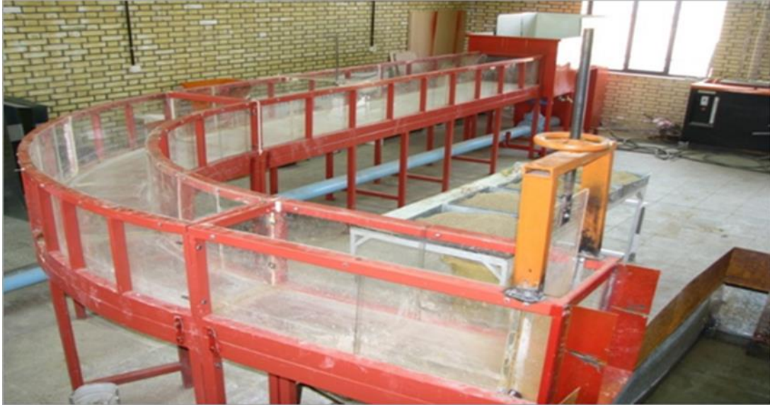
Figure 2. Experimental flume with a 90° convergent meander [24, 25]
