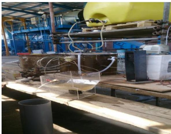
**Fig. 1. The hybrid system of activated sludge, RBC, settlement tank, and sand filter**
