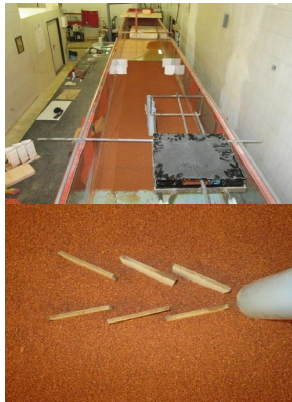
Figure 2. A view of installed pier and submerged vanes
