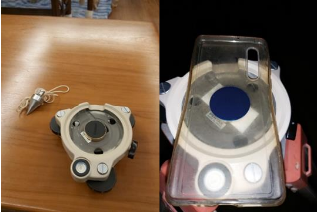
Fig. 7. Smartphone mounting on a tribrach.
