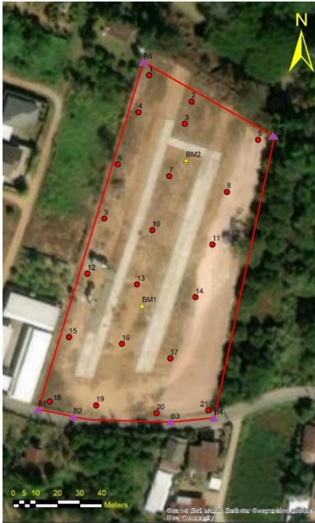
Fig. 4. Temporary ground control and testing points as well as official land marker and boundary.
