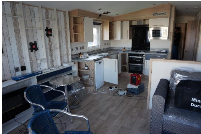
Figure 5 Electric coheating test equipment installed within one of the test caravans.
