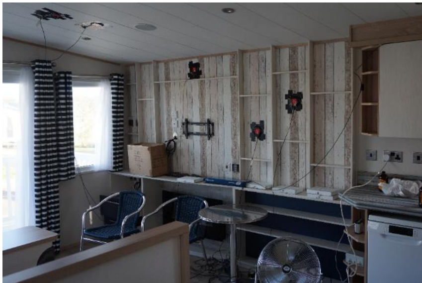
Figure 4 Location of some of the heat flux plates installed within one of the test caravans.
