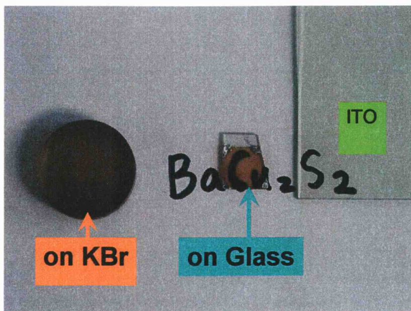
FIG. 4.5. The photograph of BaCu 2 S 2 films on glass and KBr with ITO.
