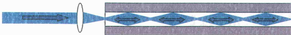
Figure 1.5 Schematic illustrating internal writing method by coupling light into the end of the fiber and relying on reflection from the end facet to set up a standing wave pattern. Note that the blue region in the fiber is not representative of the spatial distribution of the light in the fiber, but an illustration of the standing wave in light intensity.
