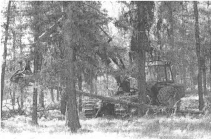
Figure 3 Rottne SMV Rapid EGS with EGS 600 harvester head, single-grip-harvester.
