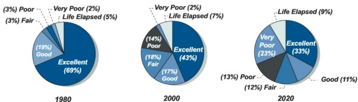
Figure 2. Estimated Sewerage Infrastructure Deterioration Trends through 2020 1
