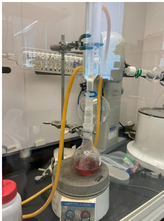
Figure 6. Reflux AuNP synthesis set up.
