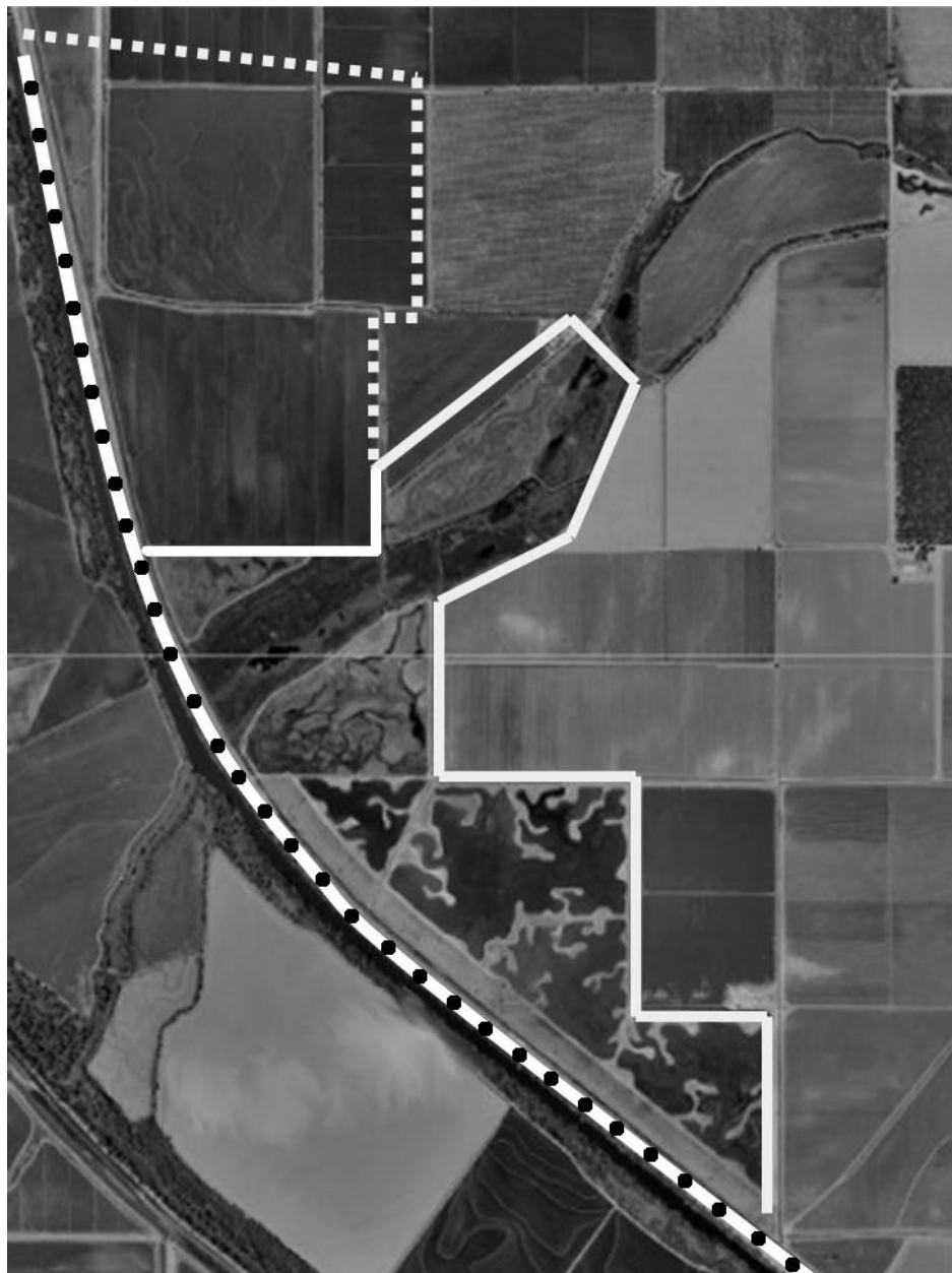
Fig. 2. Gilsizer Slough in 2006 with agricultural (rice) and constructed wetlands. The constructed wetlands are outlined by the solid line and the rice fields are outlined by the dotted line. The dashed line follows the main drainage which flows south along a levee and indicates the southern and western border of our site.
