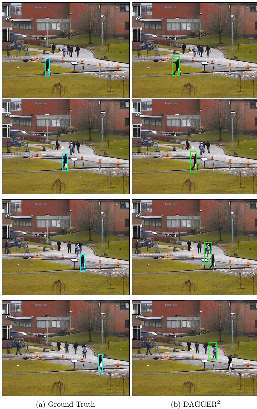
Figure 5.5: An example where even in the simple case of a person walking the GOTURN tracker loses the target, and tracks another person.
