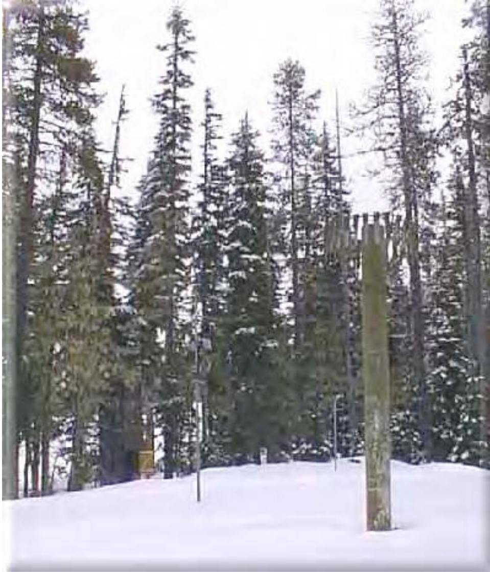
Figure 2.4: Hogg Pass SNOTEL site. The open, flat area surrounded by trees acts as a wind buffer and collects snowfall during winter. Increased solar radiation in the open area tends to accelerate snowmelt in the spring.
