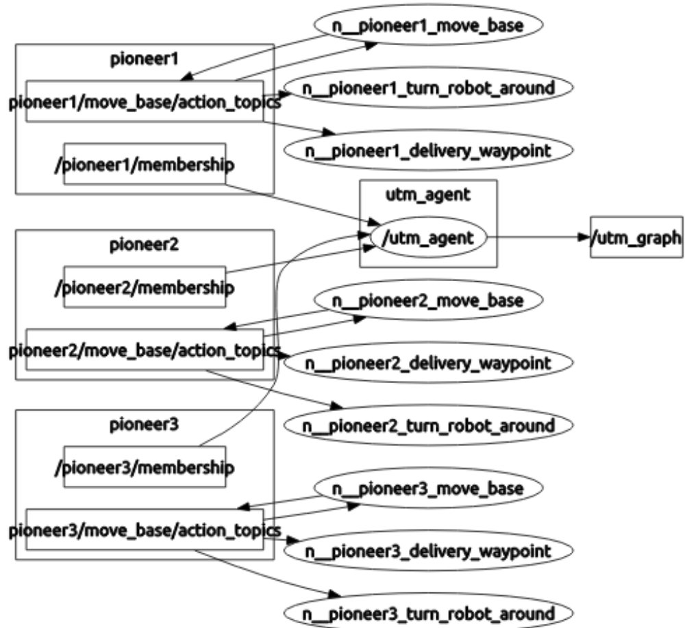
Figure 5.8: RQT graph for three pioneers in a Gazebo simulation. Pioneers communicate their position in the map with respect to which agent controls their motion (the /membership topic). This traffic information is then processed by the utm agent, which is a group of evolved neural networks. This information is then used to update the /utm_graph topic, which is the high-level cost map set by agents in the system. This is then used to update the appearance of walls for each robot topic according to its A* optimal plan.
