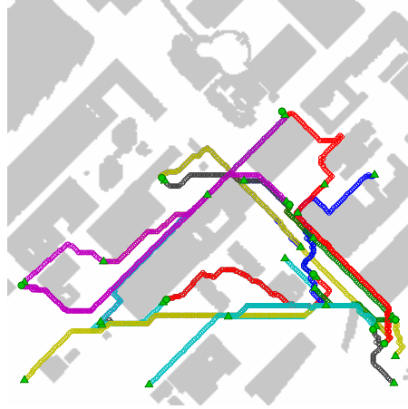
Figure 4.2: Initial planned paths for 27 UAVs in the airspace travelling from start (solid green triangle) to goal (solid green circle) locations. It can be seen that high levels of congestion may be expected in some thoroughfare regions of the airspace, such as the bottom right area where there are a group of close fixes.
