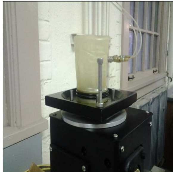
Figure 3: Assembly of specimen membrane, O-rings, and bottom platen.
