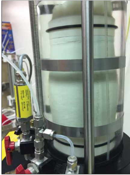
Figure 3.14: Specimen at termination of triaxial test.
