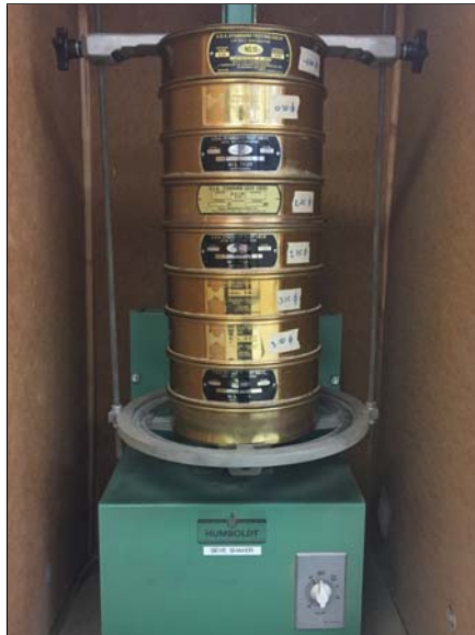
Figure 3.4: Sieve stack locked in a mechanical shaker.
