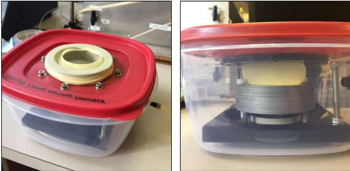
Figure 11: Membrane stretched around vacuum chamber lid fitting (left), with slight vacuum applied to chamber (right).
