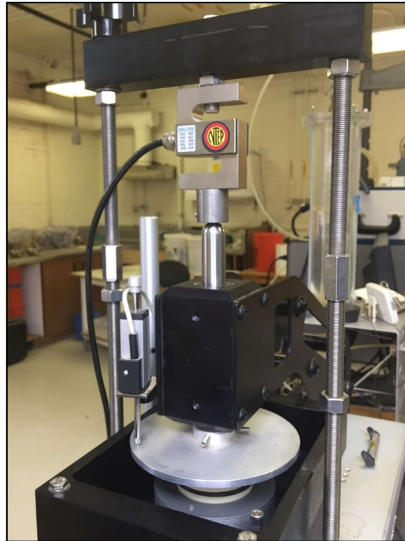
Figure 16: Shear Trac II device and specimen apparatus fully assembled.
