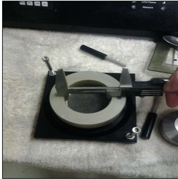
Figure 5: Membrane pulled around stacked rings with caliper to obtain inner dimensions.
