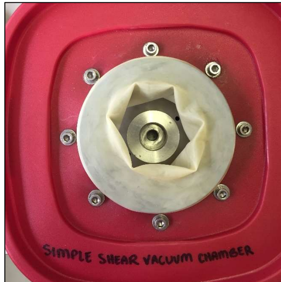
Figure 14: Top cap in place with vacuum released.
