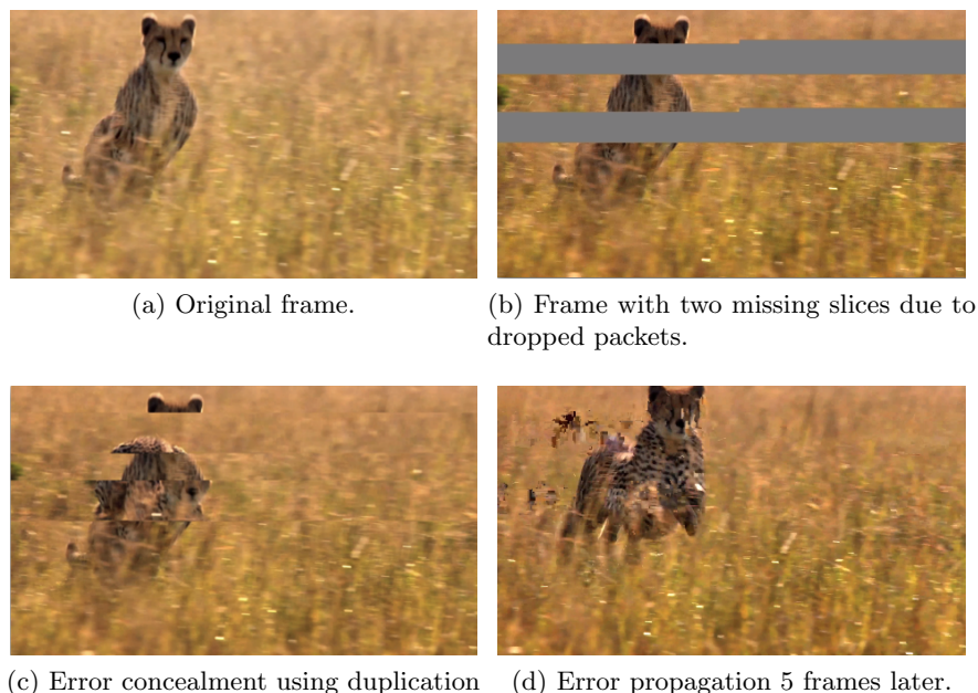
Figure 2.3: Effect of packet loss on received video.
