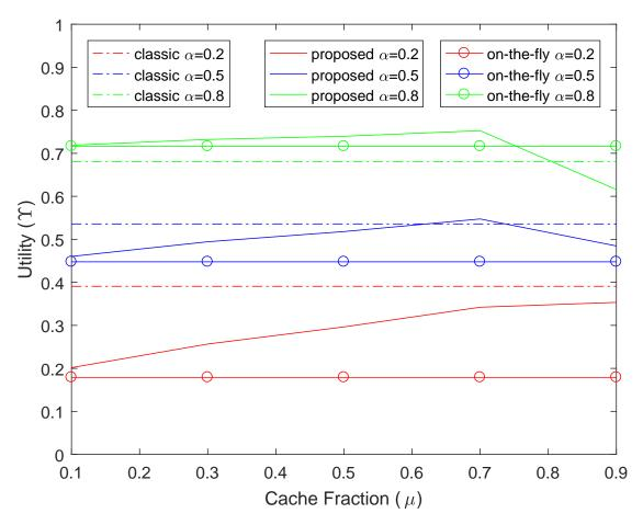
Figure 5.6: Trade off between user QoE and back-haul network load. (cache size L=30%)
