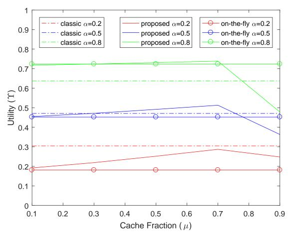
Figure 5.5: Trade off between user QoE and back-haul network load. (cache size L=20%)
