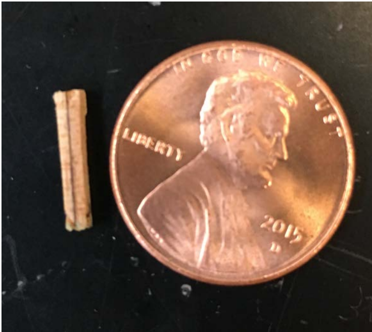
Figure 5. Micro-XCT sample with the central bondline seen as a dark line.
