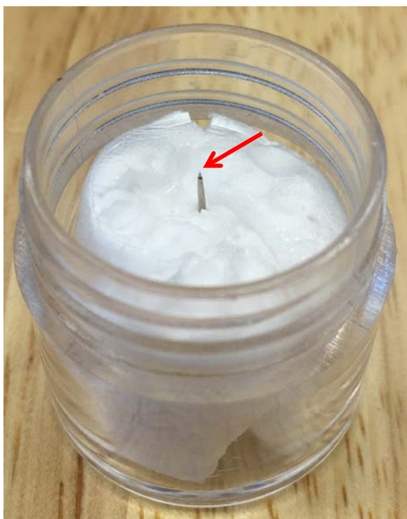
Figure 27. Mounted nano-XCT sample fixed in container with Styrofoam (arrow indicates nano XCT sample on top of needle).
