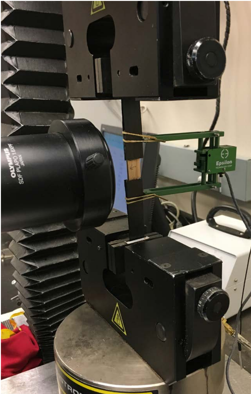
Figure 39. Verification experiment setup to test slippage and abnormal behavior in DIC and clip gauge data.
