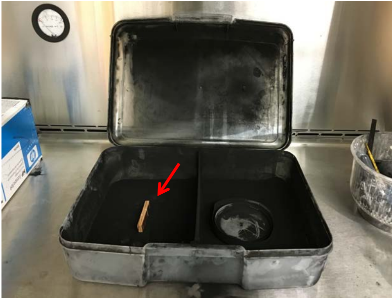
Figure 15. Air deposition speckle pattern application using ink toner; red arrow pointing at specimen.
