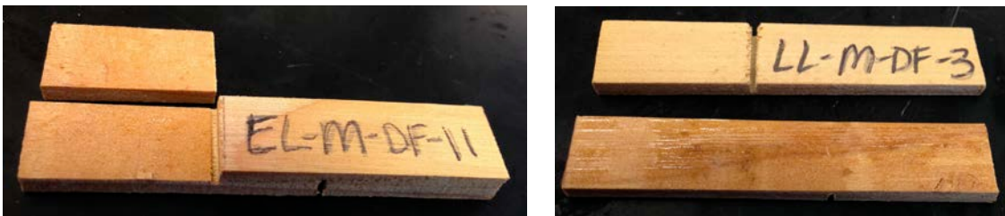
Figure 44. Two IMDI samples that delaminated during weathering cycles.
