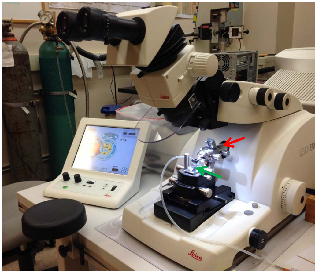
Figure 23. Leica EM UC7 ultra-microtome; red arrow indicates sample in chuck; green arrow indicates knife holder.
