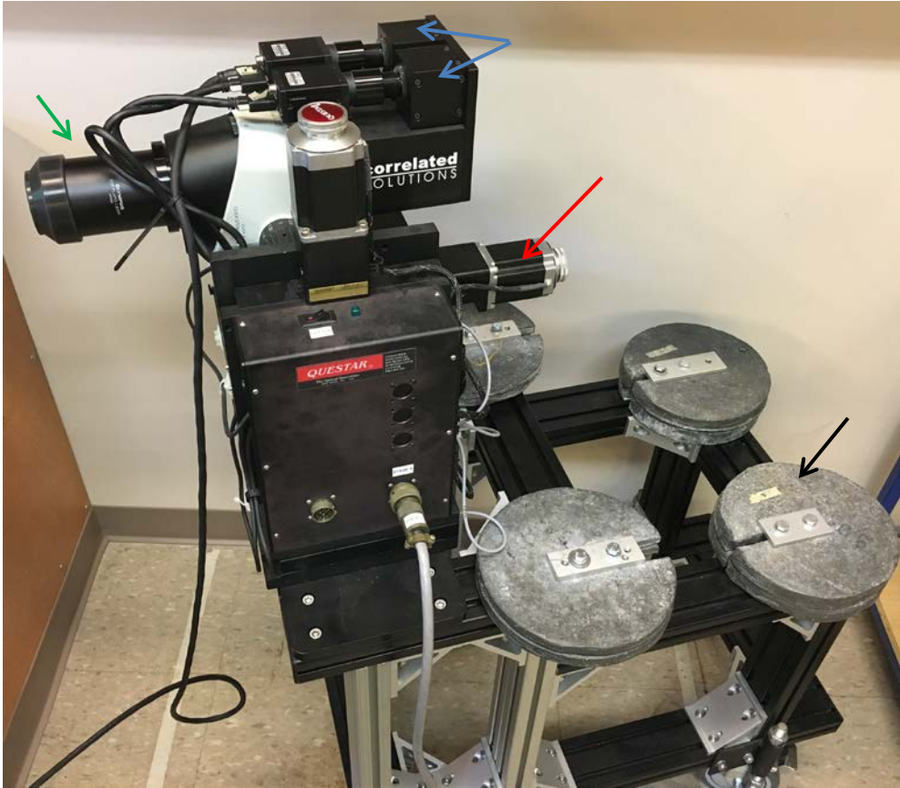
Figure 17. DIC stereomicroscope equipment on weighted cart; green arrow indicates microscope; blue arrows indicate cameras; red arrow indicates stage; black arrow indicates weighted cart.
