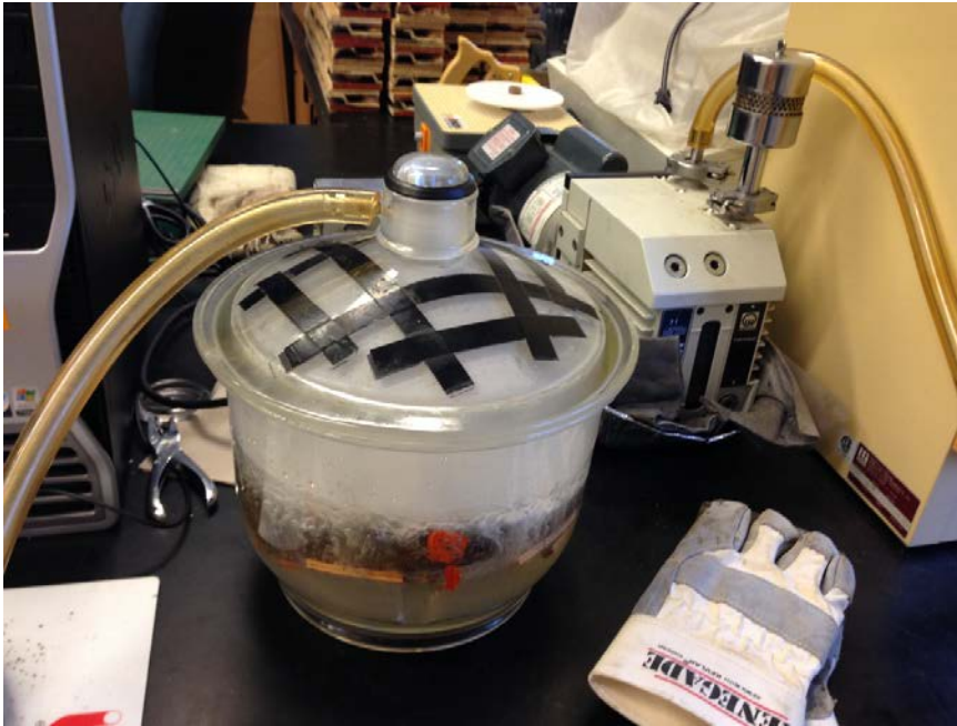
Figure 7. Desiccator used for vacuum pressure water soak on macroweathered specimens.
