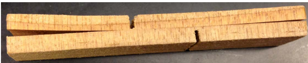
Figure 8. Example of delaminated macroweathered IMDI sample after three weathering cycles.
