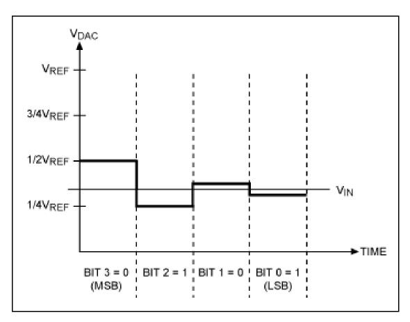
Figure 2.3: Conventional 4-bit SAR operation. [9]
