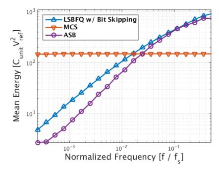
Figure 5.6: Switching energy comparison between ASB ADC, bit-skipping LSBFQ, and MCS using full-scale input.
