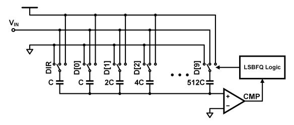
Figure 2.7: DAC architecture for a 10-bit LSBFQ ADC
