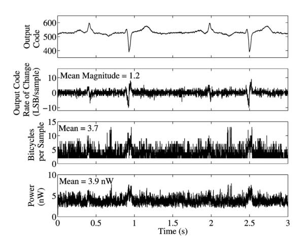
Figure 2.13: ADC response to ECG test input signal with fs = 10kHz and  $V_{DD} = 0.5V$  [12]
