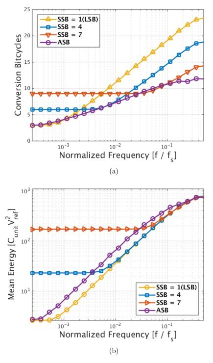
Figure 5.4: Comparisons between ASB and SSB ADC with various bits set using full-scale input for (a) mean bitcycle and (b) switching energy.
