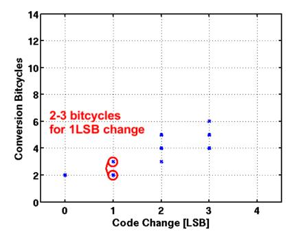
Figure 3.4: Number of bitcycles required as a function of  $\Delta D_{out}$  in a 10-bit quantizer with input frequency of  $10^{-3} f_s$ , for bit-repeating LSBFQ.
