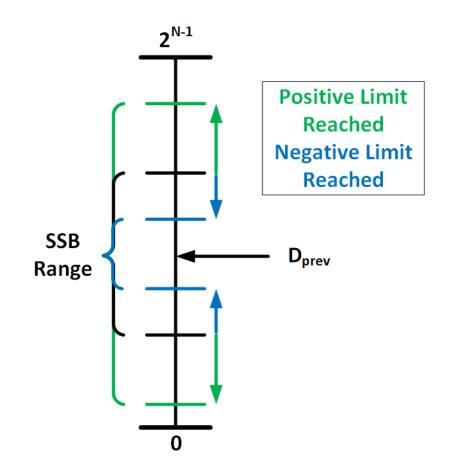
Figure 5.1: Adaptive Starting Bit ADC: feedback to adapt to the correct SSB range
