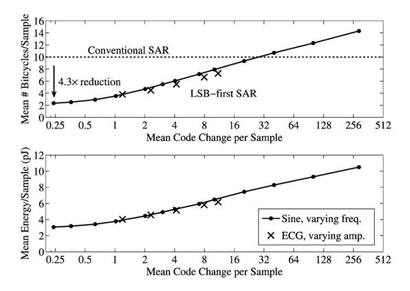
Figure 2.12: Bit-Skipping LSBFQ measured mean bitcycles/sample and mean energy consumption at fs = 10kHz and  $V_{DD} = 0.6V$  as a function of mean output code change per sample, for sine wave and ECG signals [12]
