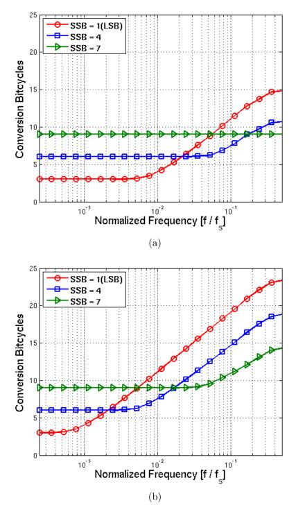
Figure 4.6: Mean number of bitcycles required by proposed algorithm as a function of frequency swept to Nyquist with various bits set as the SSB, for (a) 10% of fullscale input and (b) fullscale input.
