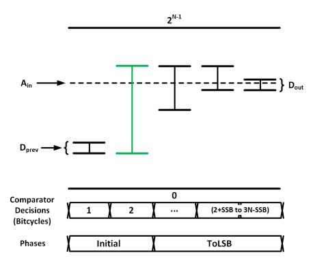
Figure 5.2: Adaptive Starting Bit ADC Operation: increasing the SSB range
