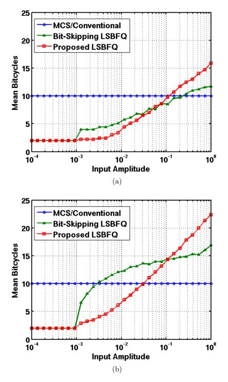
Figure 3.6: Successive-approximation bitcycles as a function of input signal amplitude, for (a)  $0.10f_s$  and (b)  $0.49f_s$ . The proposed algorithm is compared to conventional [2], MCS [5], and bit-skipping LSB-first [4] methods.
