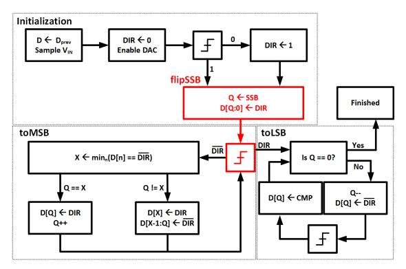
Figure 4.2: Proposed Selectable Starting Bit (SSB) algorithm.
