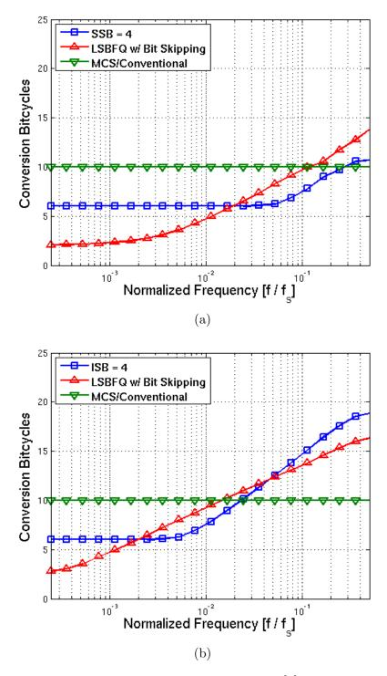
Figure 4.9: Comparisons between the SSBQ to MCS [5] and bit-skipping LSBFQ [4] for mean number of bitcycles. Comparisons are swept to Nyquist with (a) 10% fullscale input and (b) fullscale input.
