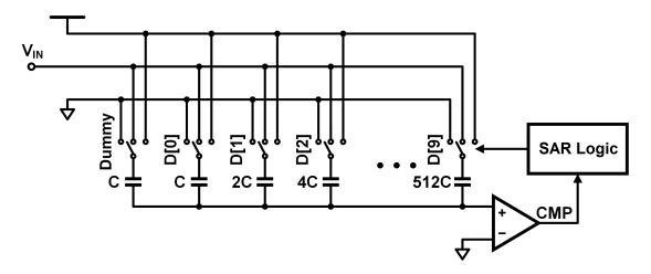
Figure 2.5: DAC architecture for a 10-bit conventional SAR ADC
