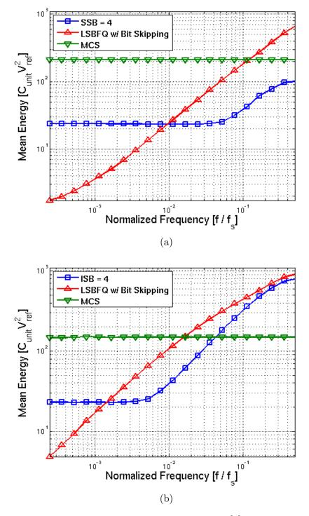
Figure 4.10: Comparisons between the SSBQ to MCS [5] and bit-skipping LSBFQ [4] for capacitor switching energy. Comparisons are swept to Nyquist with (a) 10% fullscale input and (b) fullscale input.
