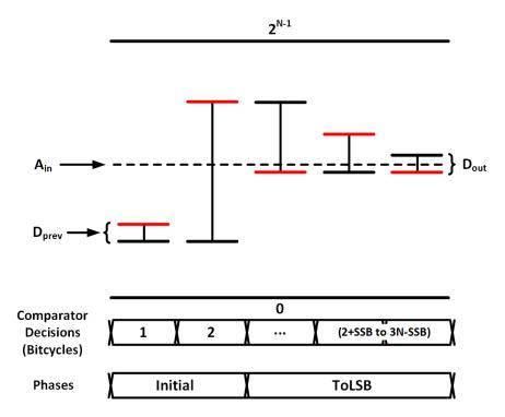
Figure 4.4: Selectable Starting Bit ADC Operation: skipping the toMSB phase
