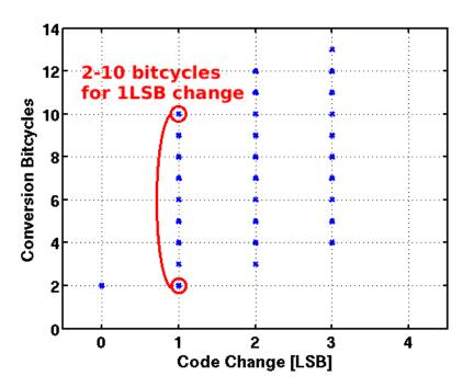
Figure 2.15: Number of bitcycles required as a function of  $\Delta D_{out}$  in a 10-bit quantizer with input frequency of  $10^{-3} f_s$ , for bit-skipping LSBFQ.
