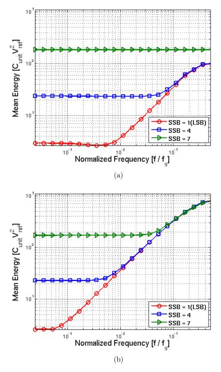
Figure 4.8: Capacitor switching energy required by proposed algorithm as a function of frequency swept to Nyquist with various bits set as the SSB, for (a) 10% of fullscale input and (b) fullscale input.
