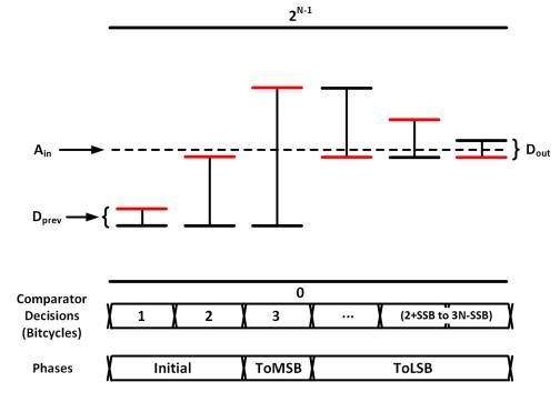
Figure 4.5: Selectable Starting Bit ADC Operation
