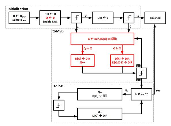
Figure 3.1: Bit-Repeating LSBFQ algorithm
