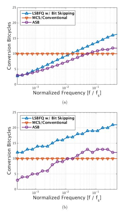
Figure 5.5: Bitcycle comparisons between ASB ADC, bit-skipping LSBFQ, and MCS using full-scale input for (a) mean and (b) max bitcycles.
