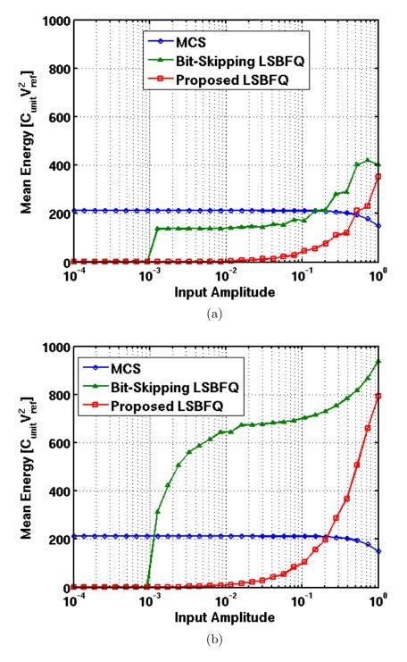
Figure 3.5: Capacitor switching energy as a function of input signal amplitude, for (a)  $0.10f_s$  and (b)  $0.49f_s$ . The proposed algorithm is compared to MCS [5], and bit-skipping LSB-first [4] methods.
