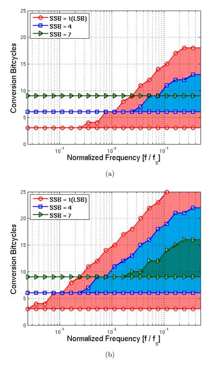
Figure 4.7: Range in number of bitcycles required by proposed algorithm as a function of frequency swept to Nyquist with various bits set as the SSB, for (a) 10% of fullscale input and (b) fullscale input.
