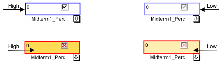
Figure 7: Output Device – Saturation of border color (top) and interior color (bottom) reflect confidence of user judgments of values being correct or incorrect.
