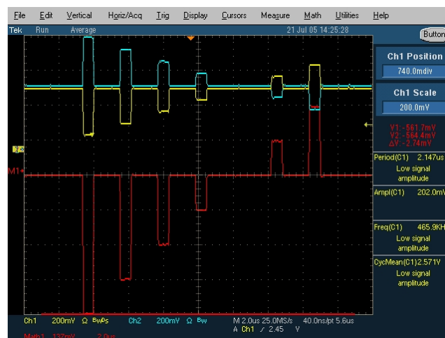
Figure 6.3: Low speed ramp. The two complementary signals and their difference.
