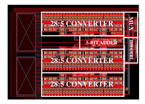
Fig. 3.12. Layout of the STDC core.
