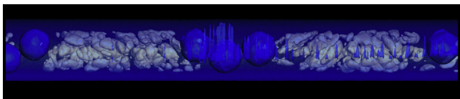
Fig. 5. A cut-away slice of the neutron tomogram of the 4.4 mm ID stainless steel pipe revealing the individual LaNi_5H_6 grains under 0.4 MPa H_2 . The blue spheres are spacers of Al_2O_3 added to the sample tube; the sample mass between spheres is 1 g, corresponding roughly 10–20 grains (sieved, particle size \geq 1.19 mm) in the initial sample preparation.
