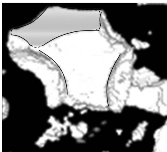
Figure 4. High-resolution (25 \mu\text{m} ) CT-image of a trapped gas bubble within 1 mm glass beads. Shown is a horizontal cut through the gas bubble, which indicates five convex curvatures.
