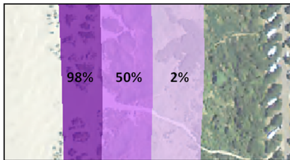
Fig. 8 Conceptual diagram illustrating the delineation of the CCHZs, which are defined probabilistically based on the 95 % confidence interval (CI) for the cross-shore distribution of expected coastal retreat distances
