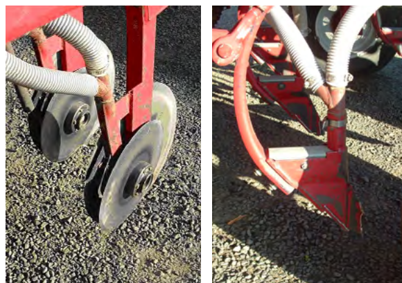
Figure 3. The customized plot drill had 13.5-inch-diameter, double-disc blades (left) mounted on a separate gang in front of narrow, hoe-type seed openers (right) on 12-inch row spacing.
