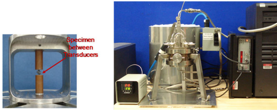
Fig. 2. High-temperature RUS chamber capable to 400°C.
