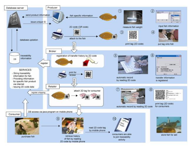
Figure 1. Proposed traceability system using 2D code.
