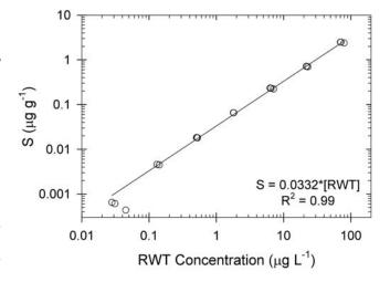
**Figure 4.** Rhodamine WT (RWT) sorption isotherm for WS03 streambed sediments (<2 mm size fraction), where S is the sorbed mass of RWT per mass of sediment. Three replicates were run for each RWT concentration value. Resulting  $K_d$  value is 0.0332 L g<sup>-1</sup>.
