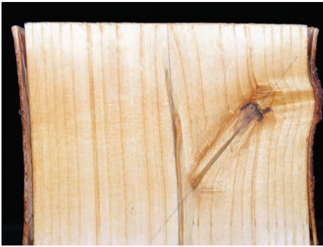
Figure 3—Stem section from tree pruned as part of the branch collar wounding study. Clear wood was produced after only 2 years following pruning.
