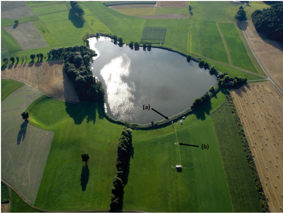
Fig. 1 Aerial photograph of the experimental site; the wind direction is computed using the two indicated sonic towers (a) and (b), and humidity measurements are taken between these two towers using the EPFL Raman lidar
