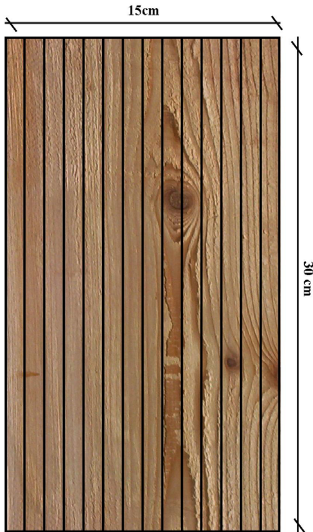
Figure 5. Cutting diagram for the penetration samples showing the widest face of the treated cedar block and the location of the cuts to produce 10mm thick strips. The dissection of the samples in this manner allowed for the assessment of preservative penetration into the insect galleries through the sample.
