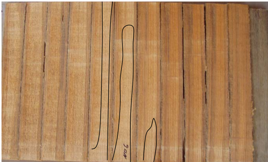
Figure 8. Example of penetration of the ClearWood MW1 treatment in western redcedar showing that chemical penetrated the entire cross section in a majority of the samples regardless of the presence of insect galleries. Areas within the black lines were not penetrated with ClearWood MW1.
