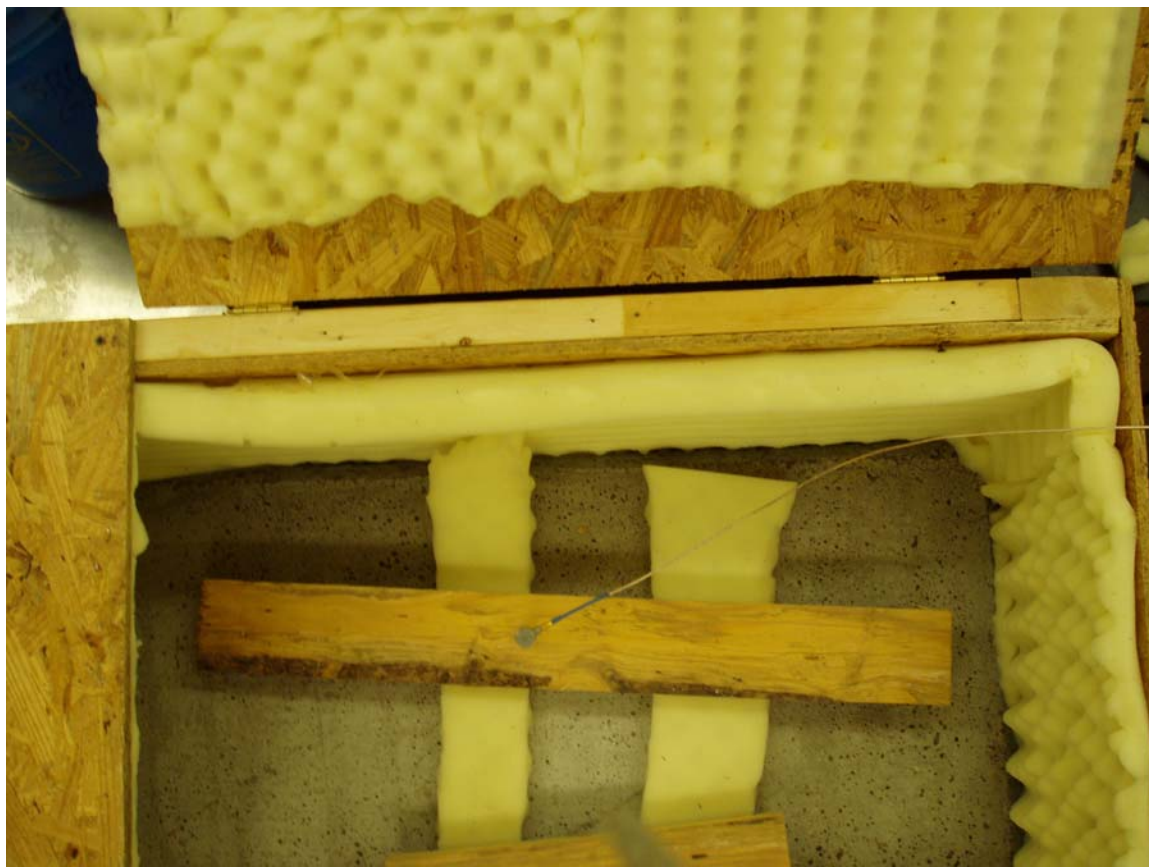
Figure 1. Interior of the acoustic sampling chamber with an insect infested board in place. The bottom of the sampling chamber consisted of cement to reduce ambient vibrations while the walls were lined with egg carton foam to dampen exterior noise.
