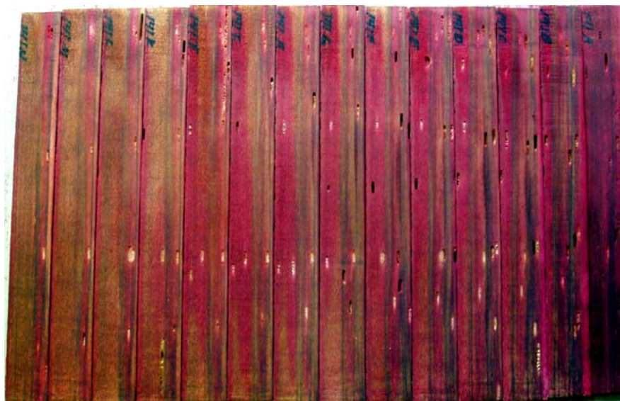
Figure 7. Example of boron penetration of western redcedar with T. blondeli galleries. The red areas indicate the presence of boron after an indicator has been applied. A majority of the insect galleries were penetrated by the chemical and chemical diffused away from the penetrated galleries in the longitudinal direction, increasing preservative coverage.
