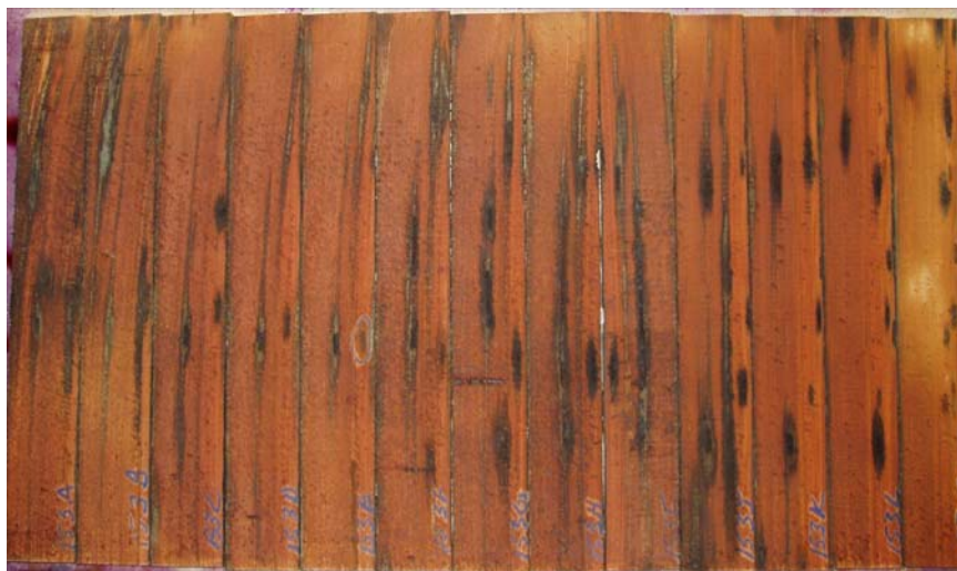
Figure 6. Example of ACQ penetration in western redcedar with T. blondeli galleries. The black color was caused by a reaction between Chrome Azurol S and the copper component of ACQ indicating that a majority of the galleries were penetrated by the preservative. Note that the chemical did not diffuse away from the galleries.
