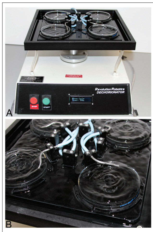
Figure 1. A modified shaker platform-based instrument for the automation of chorion removal from zebrafish embryos at 4 h postfertilization. (A) A frontal view of the modified Belly Dancer shaker. The custom machined and anodized aluminum plate is at top and holds 4 \times 100 -mm glass dishes. The control panel consists solely of a start-and-stop button and a small LCD status display. (B) A closer view of the shaker platform during a rinse phase of chorion removal. Embryos are visible in the plates. The rinse water is pumped via the onboard pump from an offboard heated source and delivered via the hose and nozzle assembly to gently overflow the plates and not suspend the embryos. The rinse water is channeled to a drain port at the rear of the platform. Agitation and pump control are via the custom onboard microcomputer.
