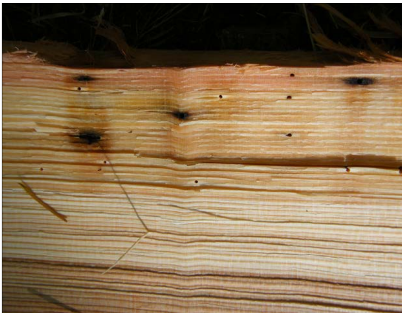
Figure 8. Pinhole borer (ambrosia beetle) galleries in sapwood. Some holes are stained with ambrosia fungi.
