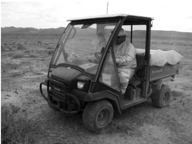
Fig. 10. Survey equipment following the release of 140 La. The two NaI(Tl) detectors were packaged in large Igloo coolers, and are next to each other, oriented side-to-side in the bed of the Kawasaki Mule. The coolers were used to limit thermal gradients; rapid temperature changes can crack NaI(Tl) crystals.
