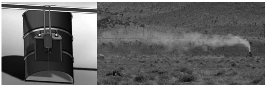
Fig. 4. Left: Cross-sectional view of the source shipping/transfer system. This image shows the system with the source extraction plug installed. Right: the PRex release occurred with surface winds of 4.5 \text{ m s}^{-1} ; the dual cone air cannon injected the ^{140}\text{La} particulate and orange smoke to 10(1) m, with the particulates introduced through the upwind cone (e.g., the particulates were riding on the upper half of the visible plume). A test run in light winds 1 wk prior to the test injected material more than 40 m into the air.
