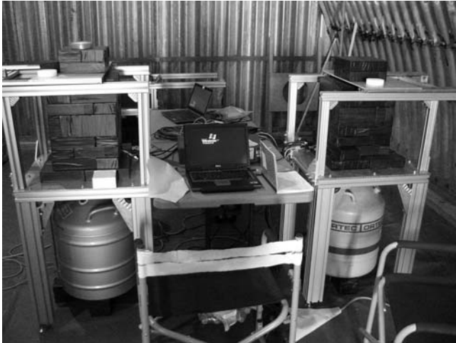
Fig. 11. Two ~50% relative efficiency HPGe detectors inside of 10.2-cm-thick lead shields. These detectors are set up in the field laboratory.
