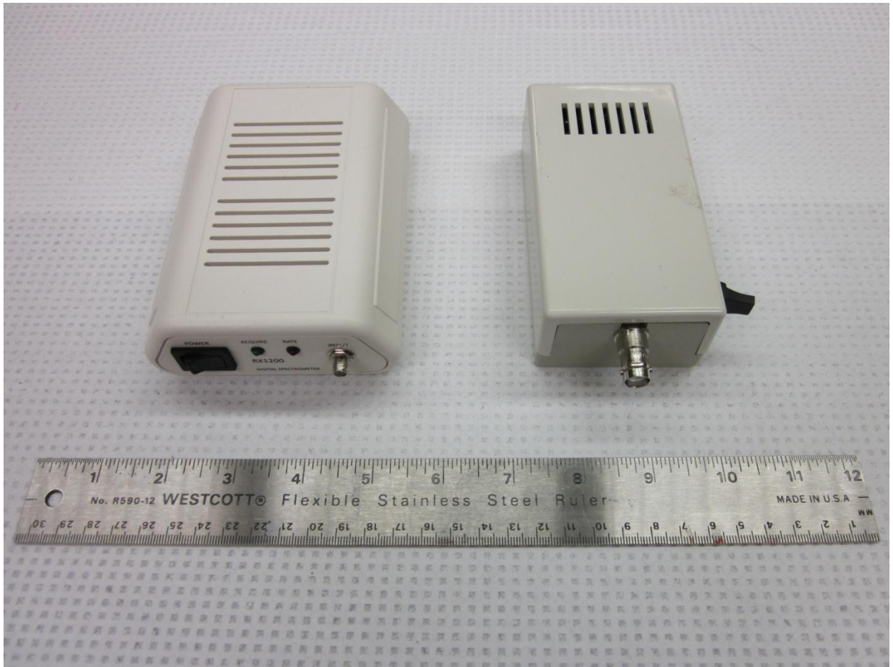
Figure 2: Avicenna RX1200 Digital Multichannel Analyzer (left) and high voltage power supply (right)
