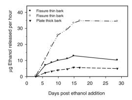
Fig. 3 Hourly ethanol release rates from a *Quercus garryana* log in the laboratory after infusing the sapwood with a 50 % ethanol solution. Three charcoal traps were used to measure ethanol release rates: two were positioned over fissures where the bark was thinner and one over a thick bark plate
