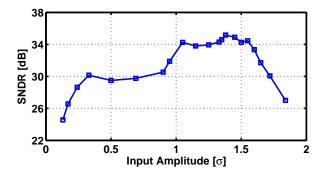
Fig. 17. SNDR from a sine-wave test as a function of input amplitude.
