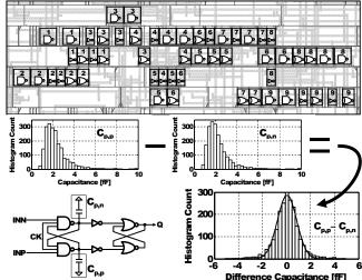
Fig. 12. Layout detail of synthesized comparator layouts and resulting systematic parasitic capacitance. The systematic variation is also found to follow a Gaussian distribution.
