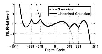
Fig. 7. A plot of the integral nonlinearity for a 2047-comparator stochastic flash ADC due to the shape of the Gaussian distribution. The remaining integral nonlinearity after applying piecewise linear approximation function is also plotted. Note that the 6-bit linear range is nearly doubled. This implies that almost twice the number of comparators lie within the "useful range" halving the number of comparators required.
