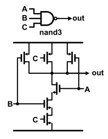
Fig. 3. A standard digital CMOS NAND3 gate and its internal transistor schematic.
