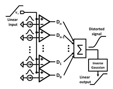
Fig. 2. A block diagram of the proposed stochastic flash ADC. The resistor ladder is replaced with random virtual references from comparator offsets. The random nature of the flash output calls for a ones adder. A inverse Gaussian CDF transformation compensates for the nonlinear distribution of the virtual references.
