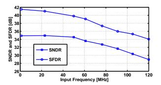
Fig. 18. SNDR and SFDR from a sine-wave test as a function of input frequency. The -3dB bandwidth at around 87-MHz is due to the RC filtering of the input network.
