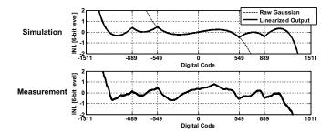
Fig. 14. Simulated and measured INL. The effect of the piecewise inverse Gaussian function can be seen to follow the expected trend.
