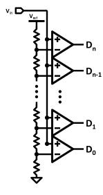
Fig. 1. A flash ADC (shown here as single-ended) is a set of monotonic references and a single comparator per reference level.
