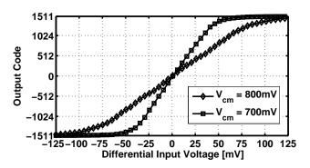
Fig. 13. Measured output transfer function of the ADC for different input common mode voltages.
