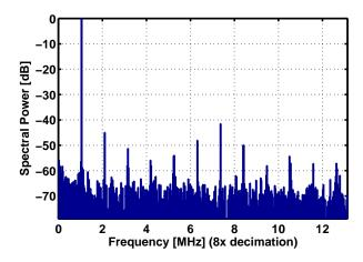
Fig. 16. Spectral plot of 1MHz input sine-wave at 210MSPS achieving 35.9dB SNDR. 8x decimation was used.
