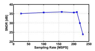
Fig. 15. Measured SNDR from a sine-wave test as function of sampling rate. The abrupt cliff at 210 MSPS is due to setup time violations occurring in the digital logic.
