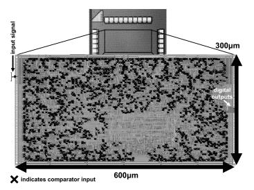
Fig. 11. Screen capture of the prototype IC with the comparator inputs each marked as a black x. The input network is automatically routed with default routing options to demonstrate true digital synthesizability. Practical implementations would direct the router to reduce the RC-delay of the input network. Dimensions are  $300\mu m$  by  $600\mu m$ .
