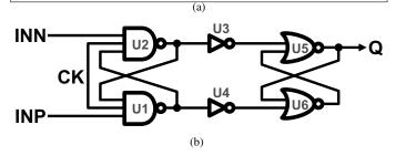
Fig. 5. a) Verilog module 'comparator' which implements a NAND3 based comparator (lines 6-11). Inverters buffer the comparator output to a SR-latch. This is to remove any memory effect caused by the latch. b) Gate-level schematic representation of the code.
