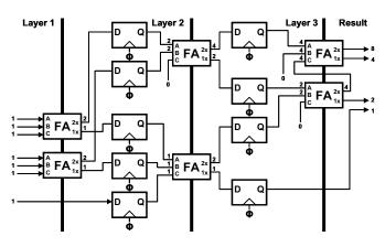
Fig. 9. Diagram of a pipelined Wallace tree ones adder for 7 inputs. D-flip-flops add latency in exchange for increasing the allowable throughput.
