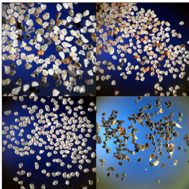
Figure 3. The four different particles studies in this work. (top left) From Satluj River, India; (top right) Paria river, Colorado, USA; (bottom left) aeolian particles provided by USGS; and (bottom right) ground coffee. The Satluj particles are most angular, and the aeolian particles are most rounded. Flakes in coffee grounds result from grinding, and could not be removed. Note the general absence of platy or elongated particles. PTI particles are similar to Paria river particles.
