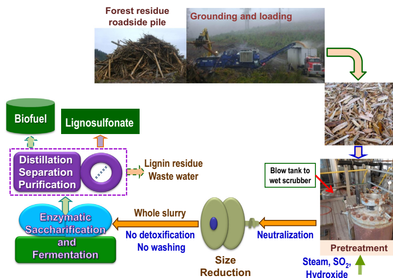
Fig. 2. A schematic process flow diagram shows Douglas-fir forest residue grinding, transportation, pretreatment and downstream saccharification and fermentation. Process boxed by dashed lines was partially conducted.
