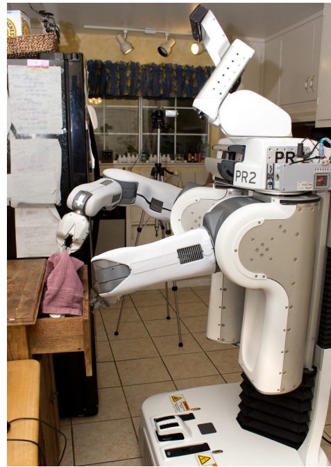
Fig. 4: Henry operating the PR2 robot to perform a remote manipulation task in his home with the Interactive Manipulation interface.
