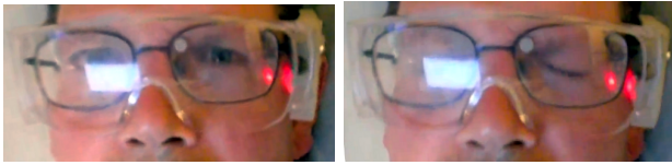
Fig. 14: Henry voluntarily winces while wearing a prototype device named the Wouse that is designed to detect wince gestures in order to stop assistive robots.
