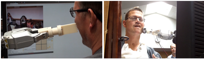
Fig. 2: Left: Henry commands the PR2 to scratch his face, and Right: to shave his cheek.
