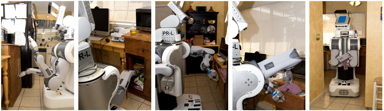
Fig. 10: Henry fetching a towel from his kitchen with the PR2. From left to right: grasping a cabinet handle, pushing open a cabinet door, opening a drawer, grasping a towel inside the drawer, and navigating to desired drop-off location.
