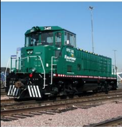
Rail Power's 'Green Goat' employs a hybrid engine.
