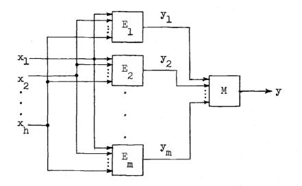
Figure 5. Redundancy of single-output elements.
