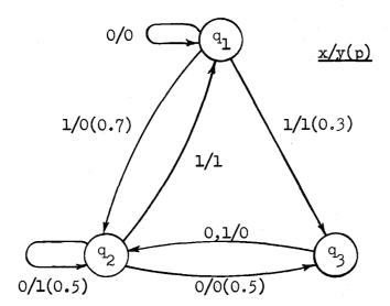
Figure 1. State graph of an SSM.
