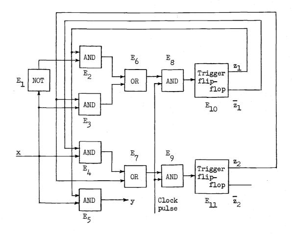
Figure 2. The sequential machine of Example 1.
