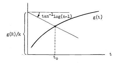
Figure 4. Graphical method for solving Inequality (40).
